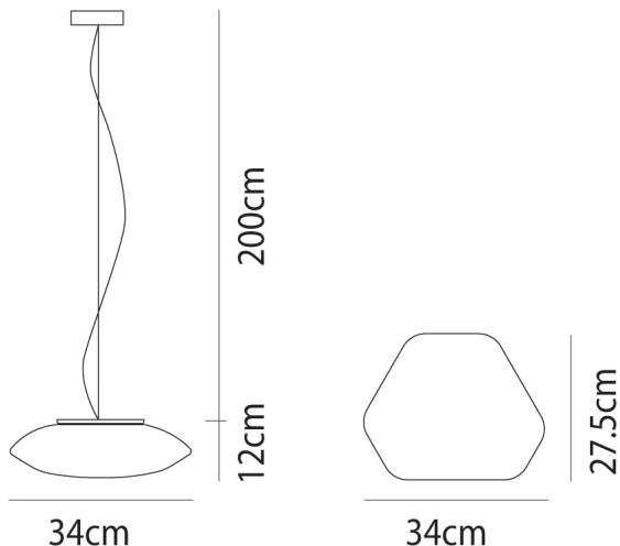
**Materials** Blown Glass**Source** 12W LED**Colour Temp** 3000K**Output** 1700lm**IP Rating** IP20**Dimming** PHASE CUT
