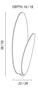
Materials 20W LED Aluminium Source **Colour Temp** 2700K Output 1920lm CRI >90 Emission Indirect TRIAC Notes Dimming Overall Dimensions: 50cm x 28cm x 18cm
