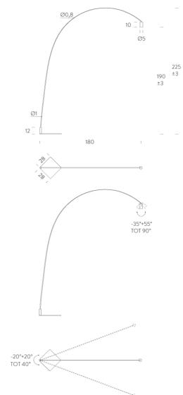
**Weight** 8kg**Materials** Aluminium**Source** 15W LED**Colour Temp** 2700K**Output** 839lm**CRI** 90**Emission** 40 degree beam, orientable**IP Rating** IP20**Dimming** Push button dimmer**Notes** Dimmer on cable
